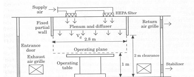
Figure 1 Typical ultra-clean ventilation arrangement in an operating theatre.
